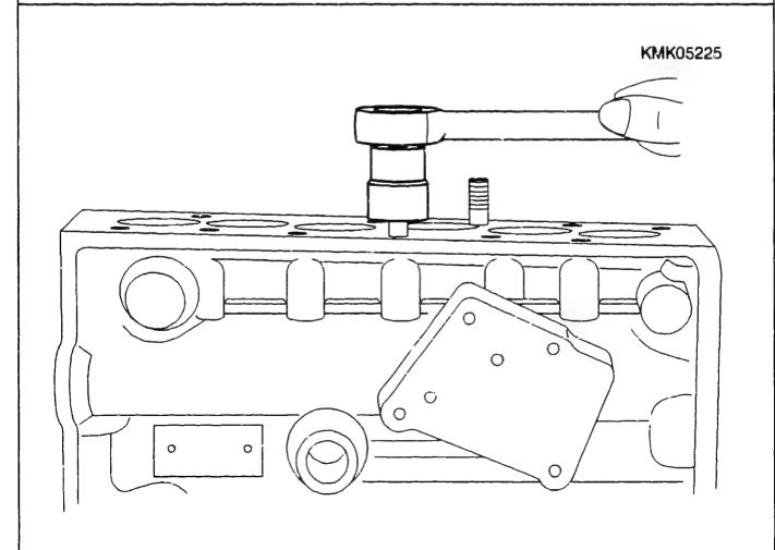
If dimension determined coincides with set value, loosen and screw off hexagon nuts.
